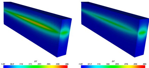
Figure 1.  $\Delta T$  (K) in Ti block 23 for swept bunches at 25 ns intervals (left) and for instantaneous profile (right). The maxima are 401 and 389 K, respectively.
