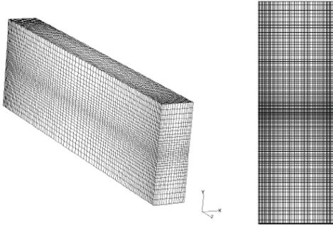
Figure 2. Simulation mesh (51200 nodes per block).
